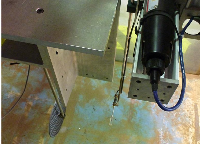
Figure 8: ADV sensor with its plastic nozzle to position the point of measurement
