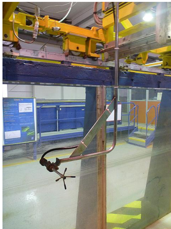
Figure 4: ADV tower support
