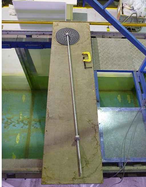
Figure 9: Porous disk fixed on a tower that is placed in front on the instrumented tower (with disk or rotor) to limit the drag force when the pump is switched on.
