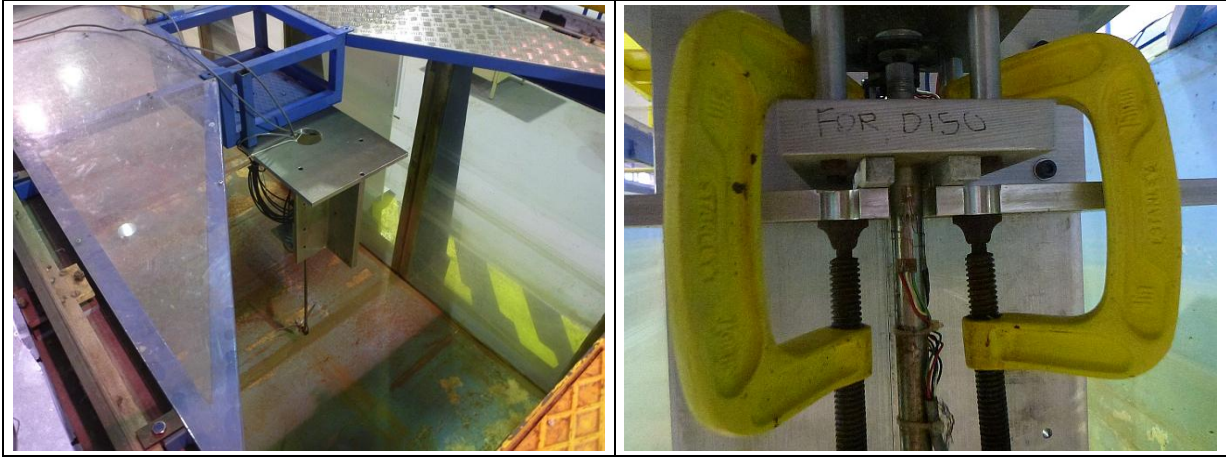
Figure 5: tower of UoM fastened to the EDF support.
