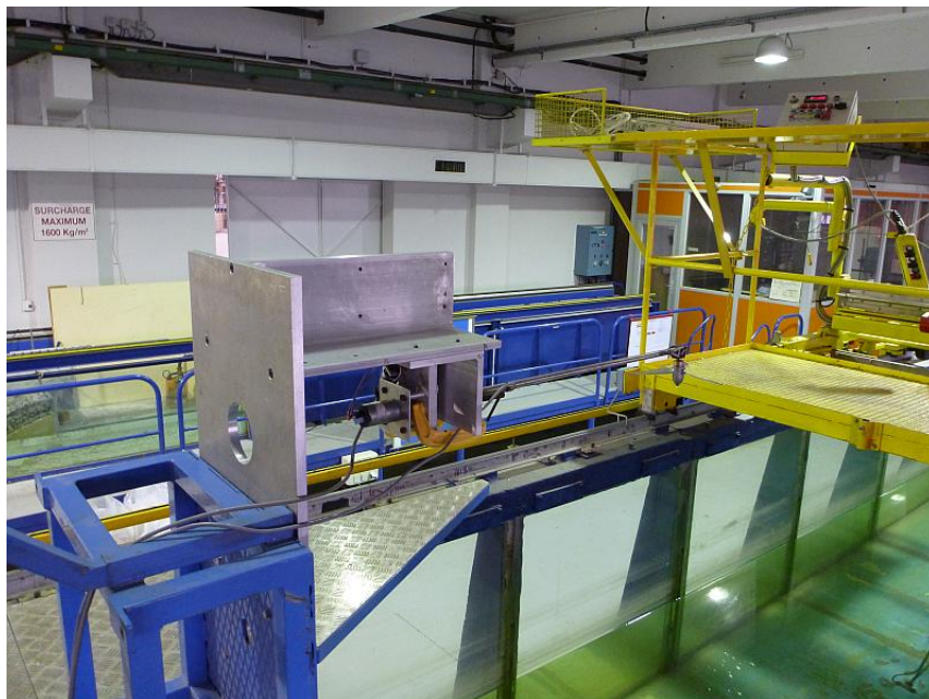
Figure 6: Rotation of the central support to place the turbine in the water
