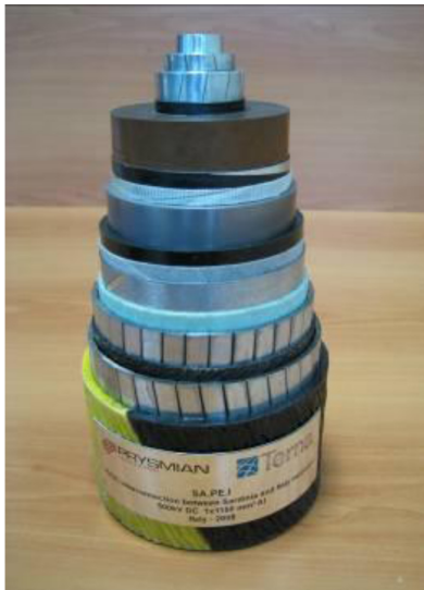
Figure 4-1 Typical submarine MI cable construction [7]
