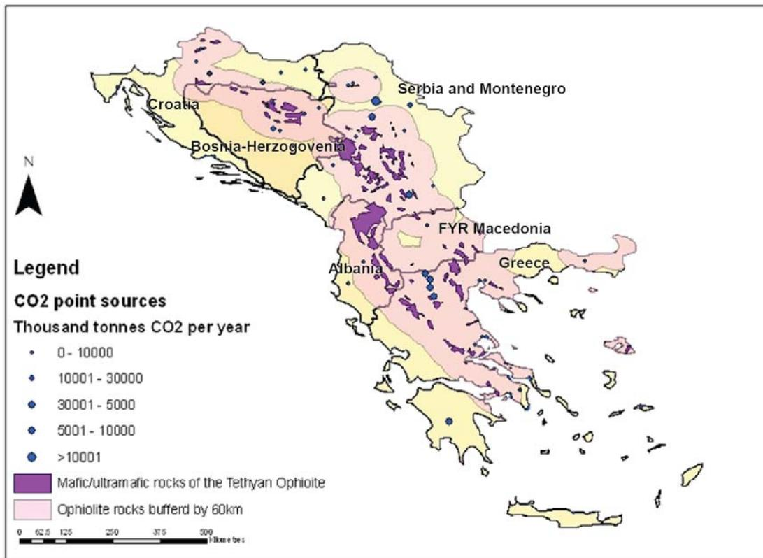
Figure 21. Ultramafic rocks and CO<sub>2</sub> emitters of southern Europe [Copyright BGS, NERC].
