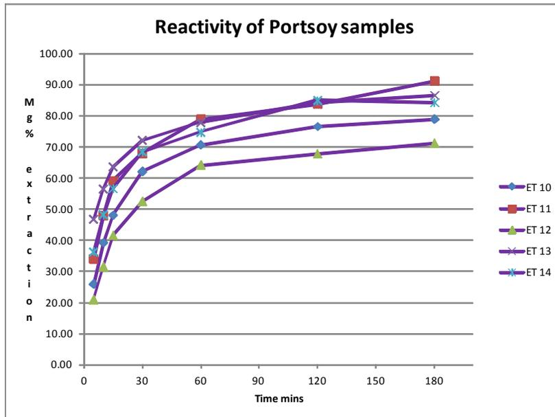
Figure 16. Plot of Mg extraction versus time for the Portsoy samples (ET 10 – ET 14).
