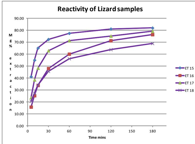
Figure 18. Plot of Mg extraction versus time for the Lizard samples (ET15 – ET 18) .
