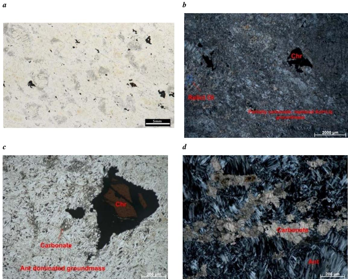
**Figure 63. Photographs of sample ET20: a) scanned polished thin section; b) crossed polarised light photomicrograph showing relict of fresh olivine and chromite within partially carbonate-replaced groundmass of antigorite and lizardite; c) plane polarised light photomicrograph showing partially altered chromite crystal within a antigorite-dominated groundmass; d) carbonate replacing serpentine minerals .**
