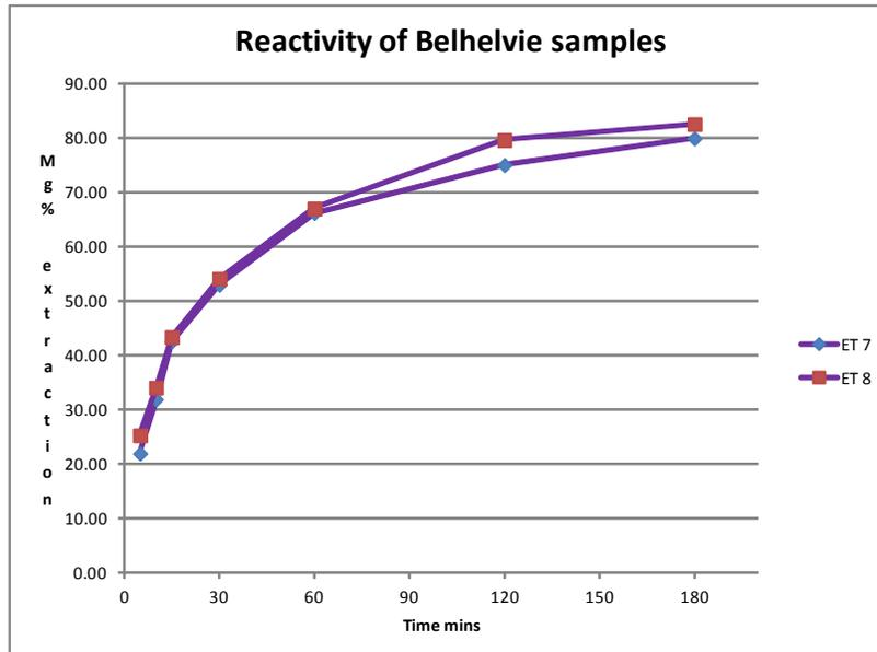
**Figure 14. Plot of Mg extraction versus time for the Belhelvie samples (ET 7 and ET 8).**
