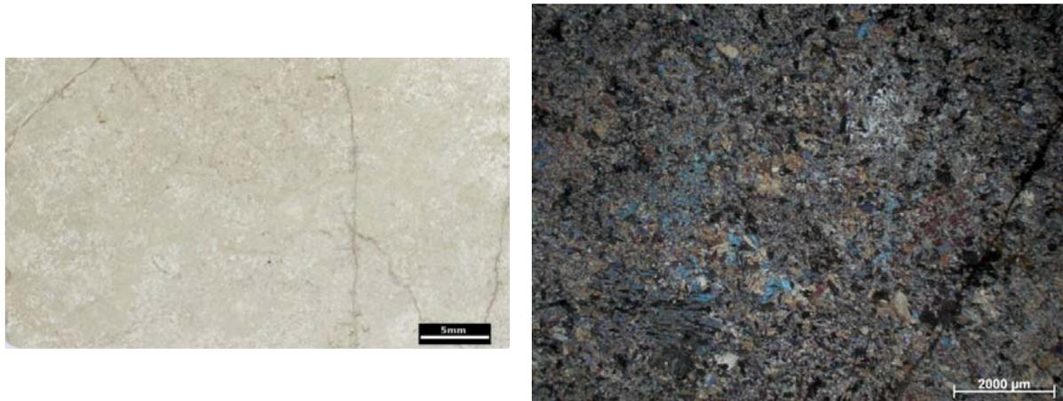
**Figure 70. Scanned polished thin section image and optical microscopy photomicrograph showing the amphibole-prehnite-rich rock .**
