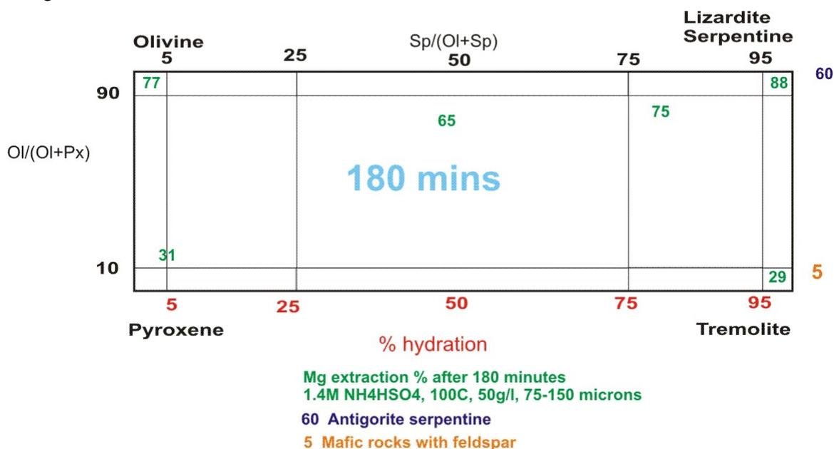
Figure 4. Extraction efficiencies of the tested ultramafic rocks in terms of composition — Reaction time 180 minutes [Copyright BGS, NERC].
