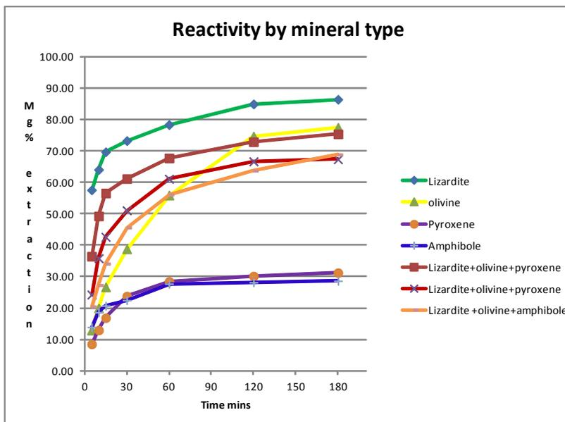
Figure 3. Plot of Mg extraction for rocks of mixed mineral compositions .
