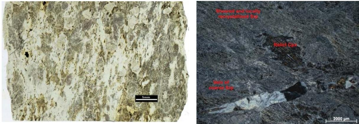
**Figure 71. Scanned polished thin section image and optical microscopy photomicrograph showing sheared and locally recrystallised serpentinite**
