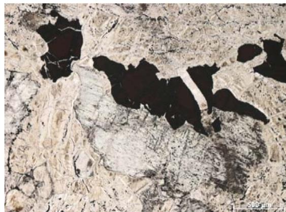
**Figure 32. Photographs of ET5 serpentinite: a) few hand specimens fragments; b) polished thin section scanned images; c) crossed polarised light photomicrograph of SL5 serpentinite with apparent bastites with mesh texture serpentine, crosscut by serpentine-infilled fractures; d) plain polarised light photomicrograph showing chromite crystals and bastite within mesh serpentine**
