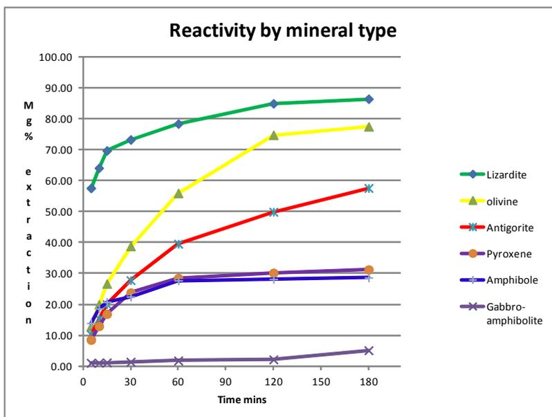
**Figure 2. The reactivity of each mineral type as a function of the extraction time using 1.4M ammonium sulphate .**
