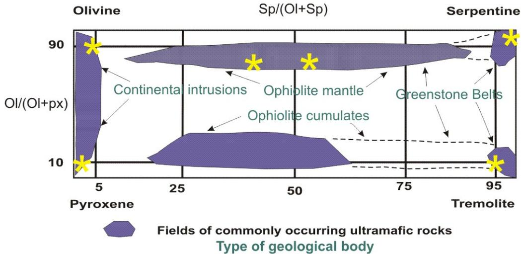
**Figure 1. The range of compositions of ultramafic rocks and the samples tested shown by yellow stars [Copyright BGS, NERC]**
