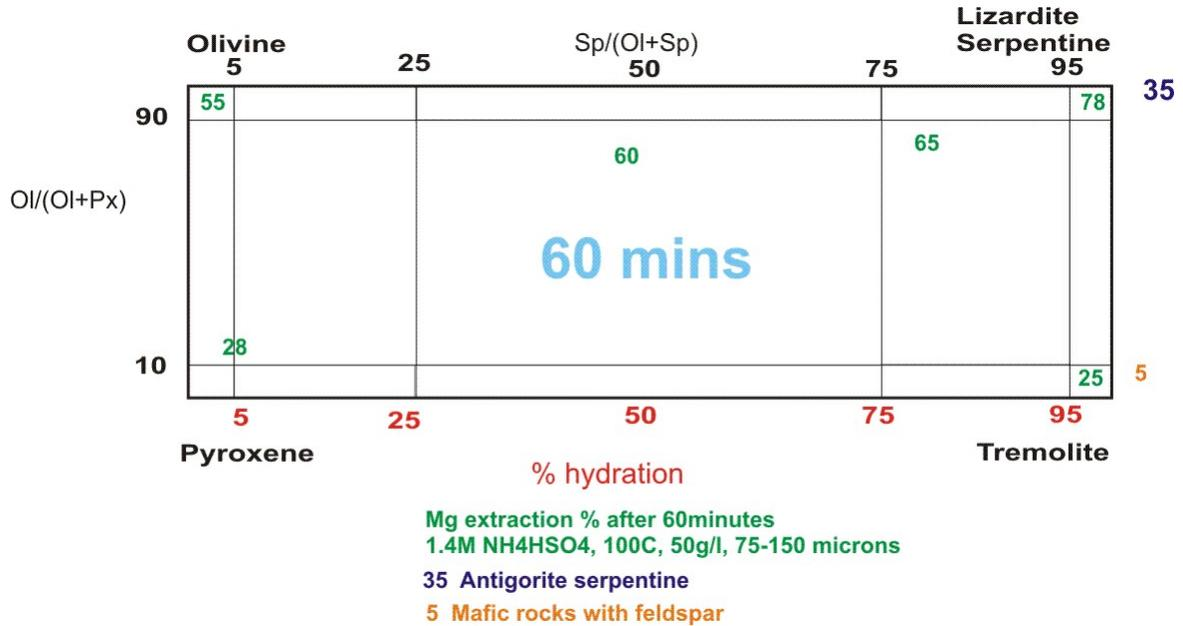
Figure 5. Extraction efficiencies of the tested ultramafic rocks in terms of composition — Reaction time 60 minutes [Copyright BGS, NERC].
