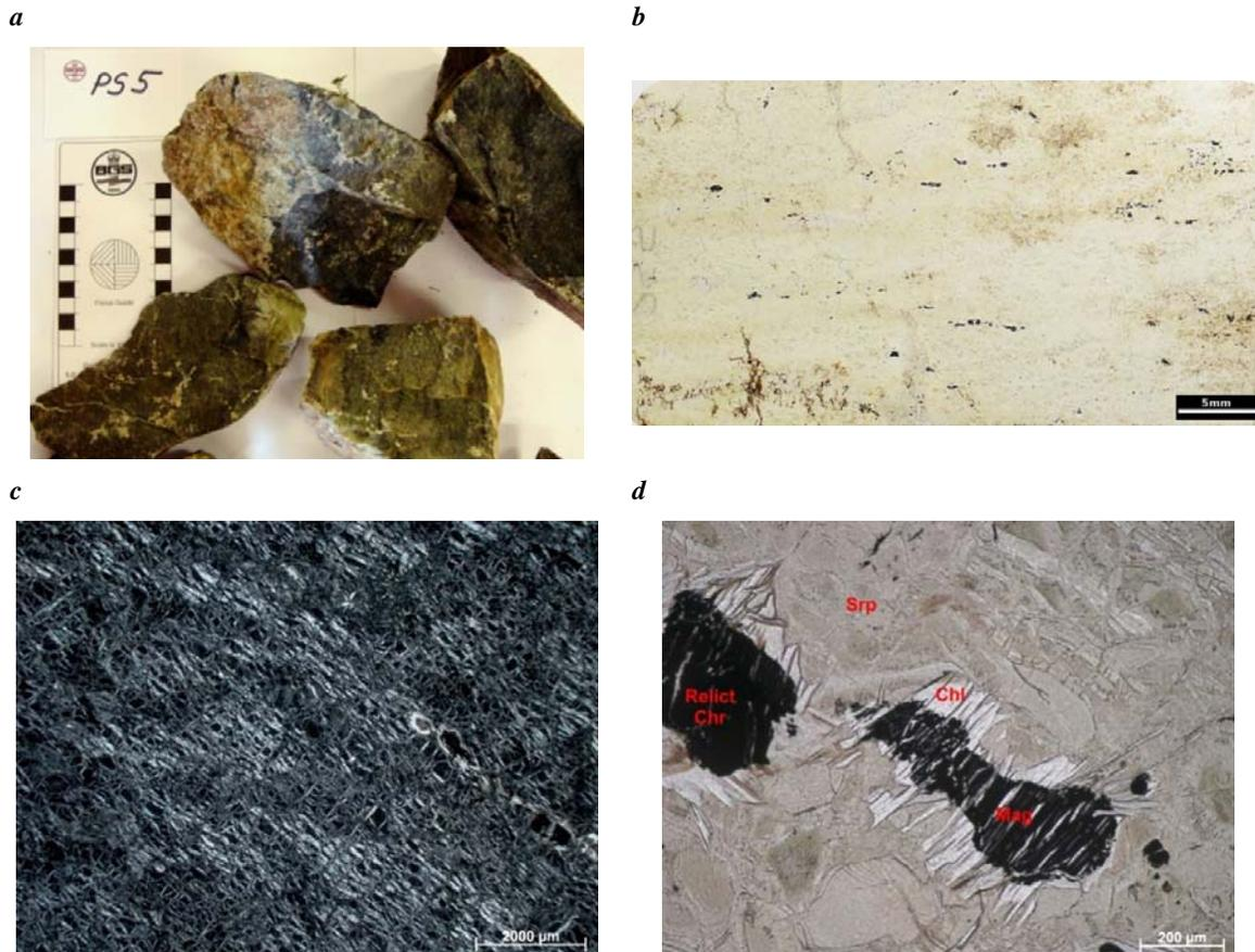
Figure 50. Photographs of sample ET13, chlorite-rich serpentinite: a) hand specimen; b) scanned polished thin section; c) crossed polarised light photomicrograph showing sheared serpentine mesh; d) altered chromite (now magnetite) and distinctive chlorite halo .
