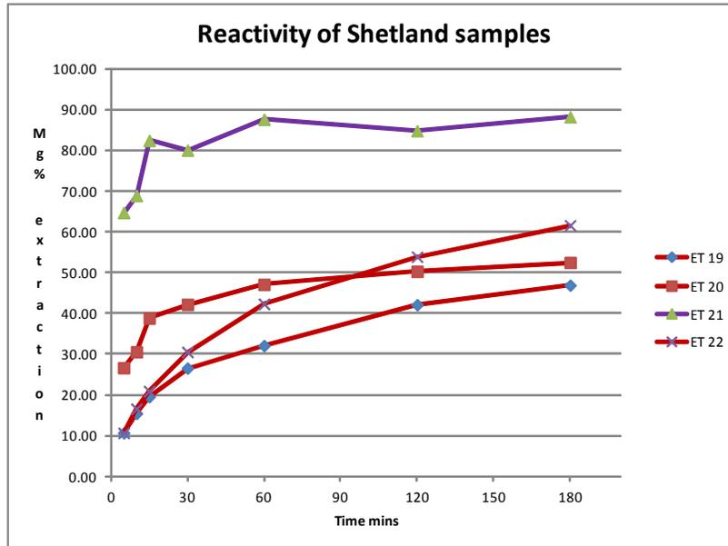
Figure 20. Plot of Mg extraction versus time for the Shetland samples (ET 19 – ET 22).
