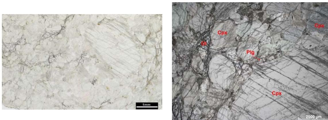
**Figure 69. Scanned polished thin section image and optical microscopy photomicrograph showing large crystals of pyroxene in association with plagioclase and olivine .**
