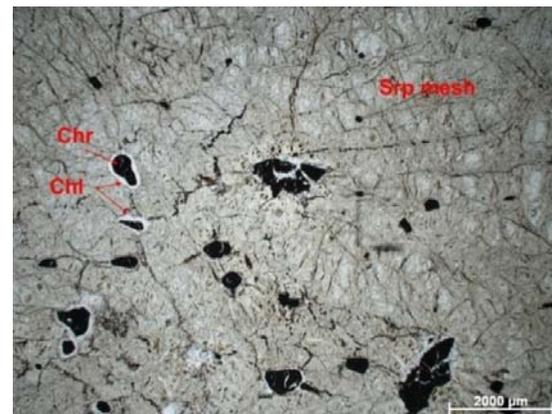
**Figure 64.** Scanned polished thin section image of the rock analysed and optical microscopy light image showing mesh texture serpentinite and chromites (black) surrounded by distinctive rim of chlorite.
