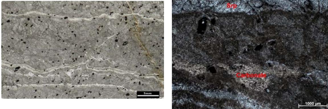
**Figure 65. Scanned polished thin section and optical microscopy photomicrograph (cross-polarized light) showing partially carbonate replaced serpentine .**
