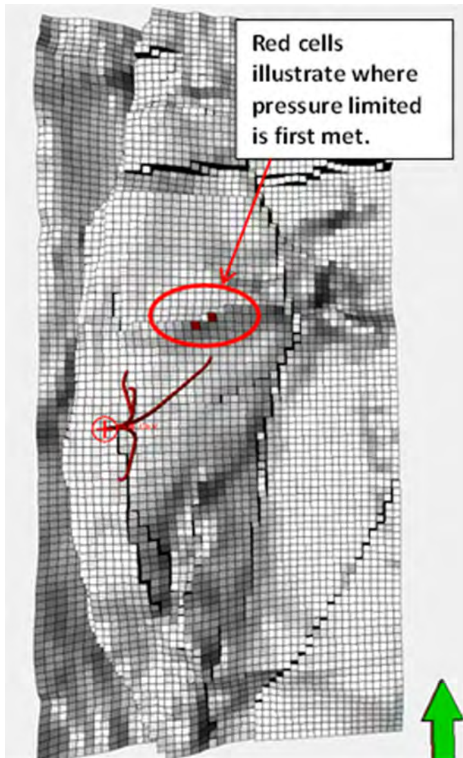
Figure 3-48 Location where pressure limit is first violated in reference case model
