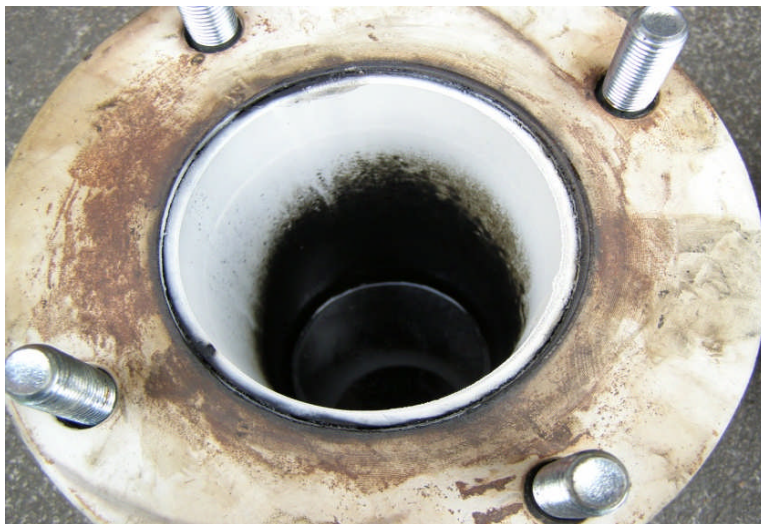
Figure 28 Downdraft Gasification (Food and Paper and Card) Cooler 4 - White Deposits
