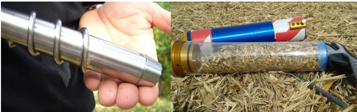
Figure 2-6: Left – image of the corer bit; right – the subsample of Miscanthus
