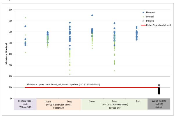
Figure 12-2: Moisture content (ar) of woody project feedstocks in comparison to historical wood pellet data and pellet standard limits
