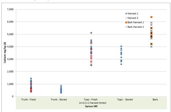
Figure 9-10: Results from the calcium analysis of spruce SRF (note – calcium in fuel is back calculated from ash oxide composition)
