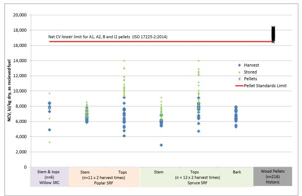
Figure 12-3: Net calorific values (ar) of woody project feedstocks in comparison to historical wood pellet data and pellet standard limits
