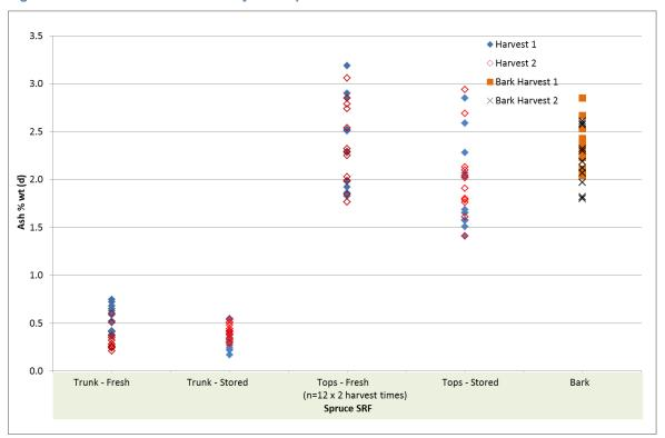
Figure 9-5: Results from the silicon analysis of spruce SRF (note – silicon in fuel is back calculated from ash oxide composition)
