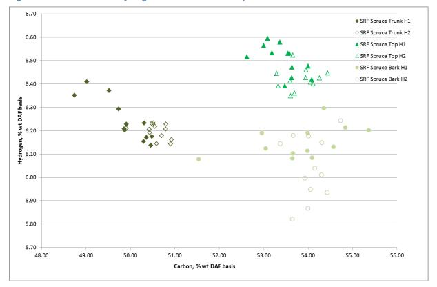
Figure 4-10: Carbon verses Hydrogen content for the SRF spruce feedstocks
