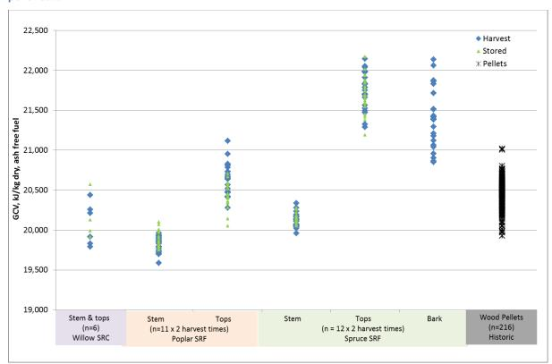
Figure 12-1: Gross calorific values (DAF) of woody project feedstocks in comparison to historical wood pellet data
