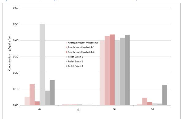
Figure 11-10: Arsenic, mercury, selenium and cadmium content of fresh and pelletised Miscanthus
