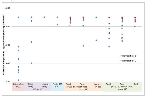
Figure 4-16: Comparison of initial deformation temperatures (reducing conditions) across all feedstocks in study 1 & 3
