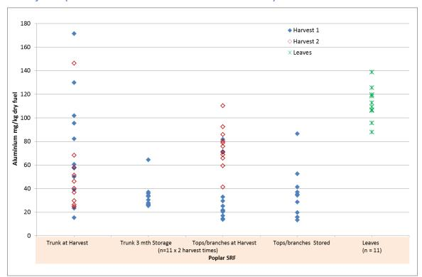
Figure 8-4: Results from the aluminium (d) analysis of poplar SRF in study 1, showing harvest time impacts in study 1 & 3 (note: back-calculated from aluminium oxide in ash)
