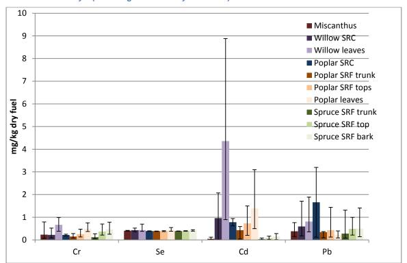
Figure 4-13: Comparison of average chromium, selenium, cadmium and lead values across all feedstocks in study 1 (data range indicated by error bars)
