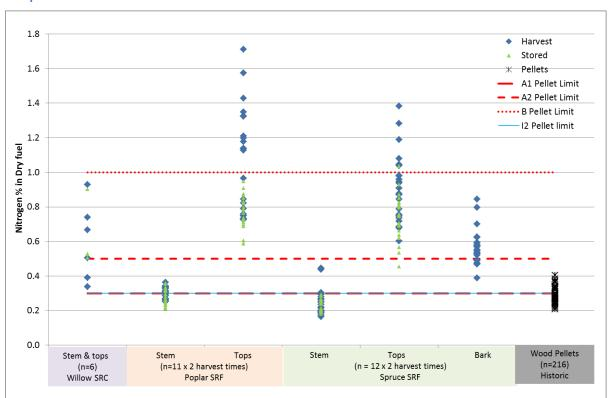
Figure 12-6: Nitrogen content (d) of woody project feedstocks in comparison to historical wood pellet data and pellet standard limits
