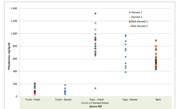
Figure 9-11: Results from the phosphorous analysis of spruce SRF (note – phosphorous in fuel is back calculated from ash oxide composition)
