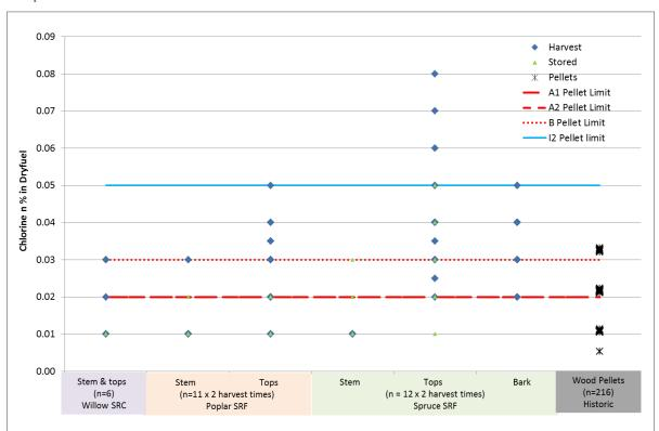
Figure 12-8: Chlorine content (d) of woody project feedstocks in comparison to historical wood pellet data and pellet standard limits
