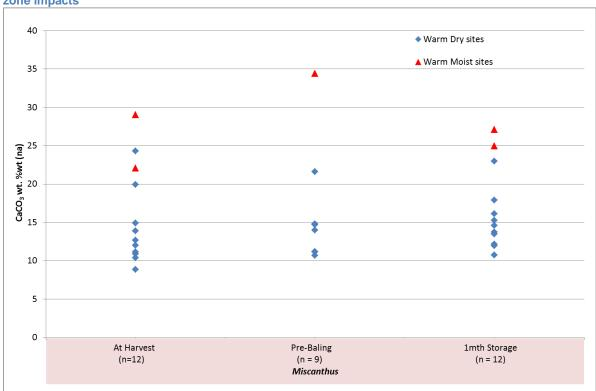
Figure 5-2: Results from the calcium carbonate in ash analysis of *Miscanthus* in study 1, showing climate zone impacts
