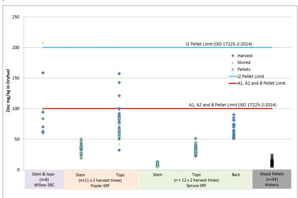
Figure 12-9: Zinc content (d) of woody project feedstocks in comparison to historical wood pellet data and pellet standard limits
