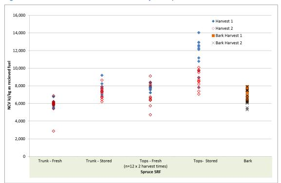
Figure 9-3: Results from the Net Calorific Value analysis of spruce SRF
