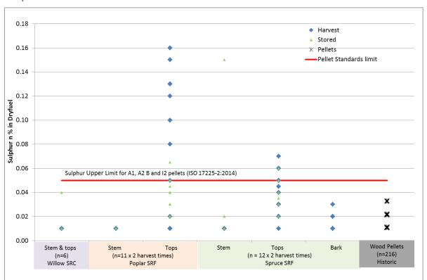
Figure 12-7: Sulphur content (d) of woody project feedstocks in comparison to historical wood pellet data and pellet standard limits
