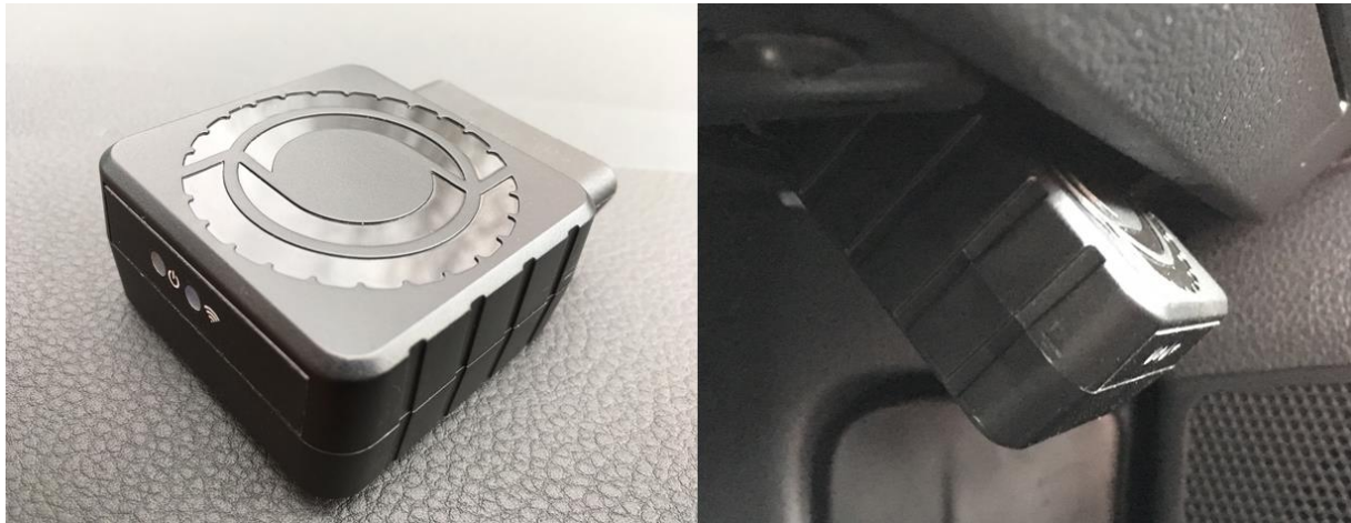
Figure 11: FleetCarma telematics dongle (left) and in situ in vehicle (right)
