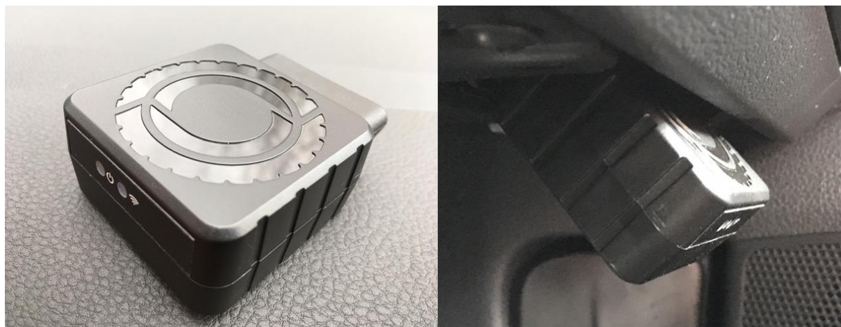
Figure 24: FleetCarma telematics dongle (left) and in situ in vehicle (right)
